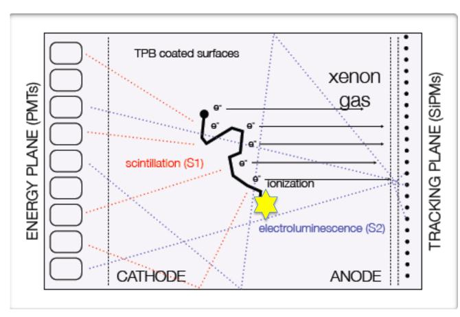
High pressure Xe TPC Enriched at 90% in <sup>136</sup>Xe Operating at 15 bar in EL mode
