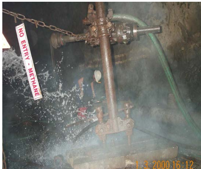
Drilling a borehole and sampling groundwater at 3 km depth in a South African gold mine.
