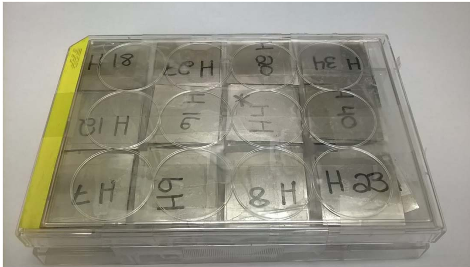
60 Co coupons irradiation “array”
