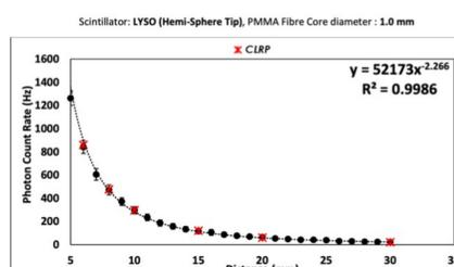
**Performance with LYSO:** since scintillation light is "compressed", the threshold could be increased reducing the DCR to ~ 4 Hz
