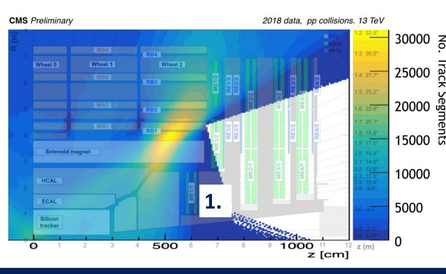
Background segments reconstructed in the MB1 chambers propagated in the z-R plane: due to calorimeter gaps and originate from conversions in the solenoid or in the iron yoke
