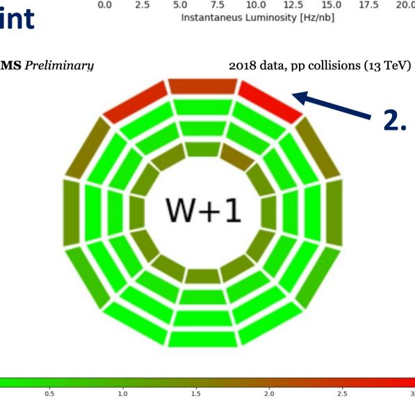
Slope of current vs LHC Luminosity
