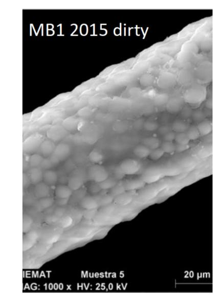
Electronic microscope scan of an extracted aged wire coated with pollutant
