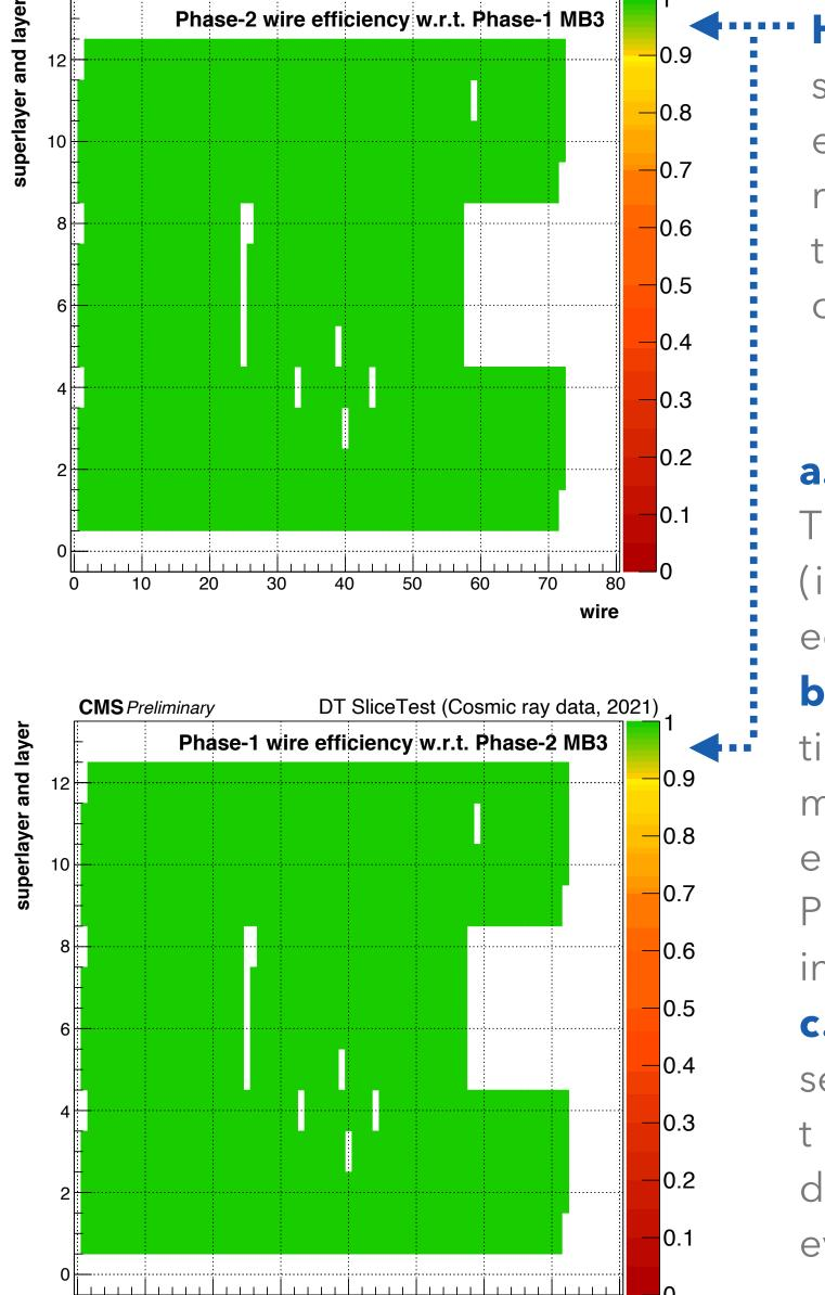
**★····· Hit detection :** tested in  $\frac{8}{2}$ several aspects. E.g. 5000 efficiency of the Phase-2 readout is probed against the one of Phase-1 for each cell (and vice-versa).
