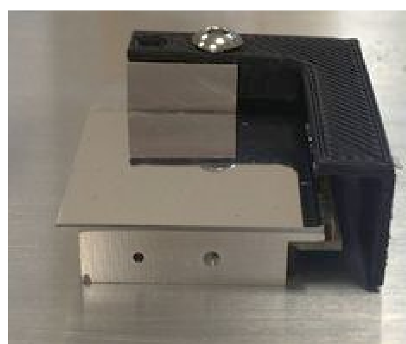
Fig.1: 500 \mu\text{m} P-type Si sensor bonded to the HEXITEC ASIC.
