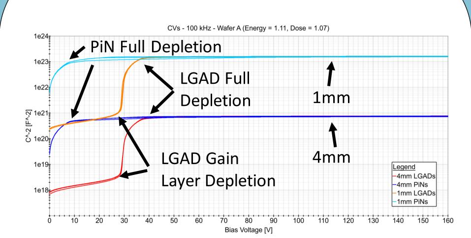
Capacitance (1/C²) vs Bias Voltage curves for 4mm & 1mm devices of a single wafer type. There is a clear capaticance difference for the difference sizes. We also see the delay in **full depletion** in LGADs due to the **gain layer depletion**.
