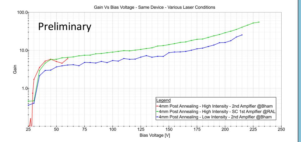
The gain is calculated as the **ratio** of the pulse integral between an LGAD and a PiN.
