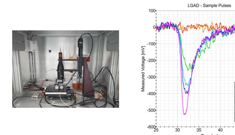
Charge is injected via a **pulsed 1064 nm laser**. The resultant pulse from the sensor (which is connected to a fast amplifier) is integrated over a specific time window. The result of that **integral**, as a function of bias voltage, can be plotted.
