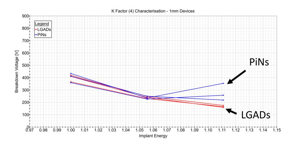
Breakdown is defined as the significant increase in leakage current as a function of bias voltage. Breakdown voltage is calculated via the **K-Factor characterisation** method, where **K = 4** is defined as "**soft breakdown**". This is then plotted against the normalised wafer implant energy.
