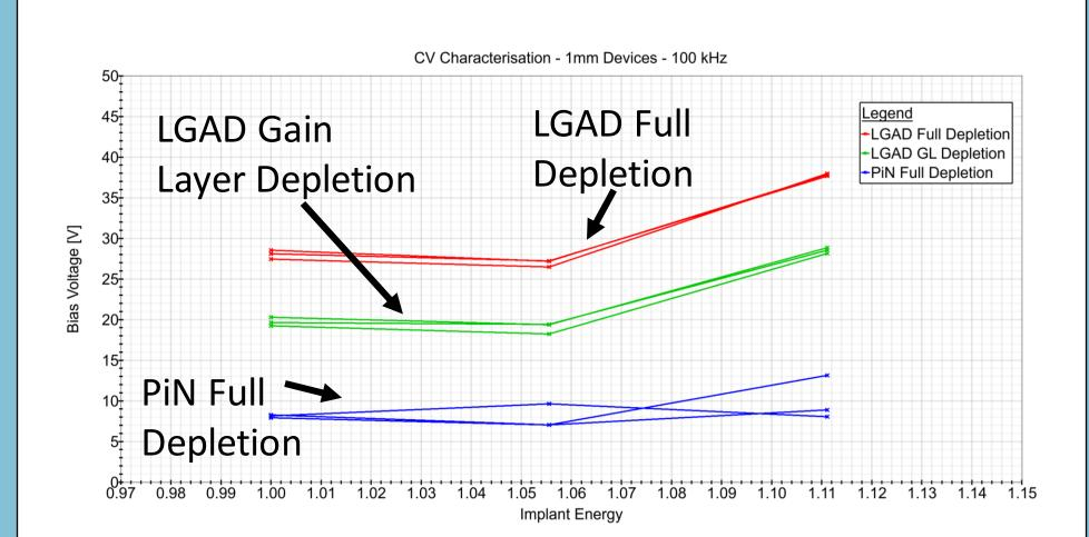
We can extract the two depletion voltages and plot them against the normalised implant energy.
