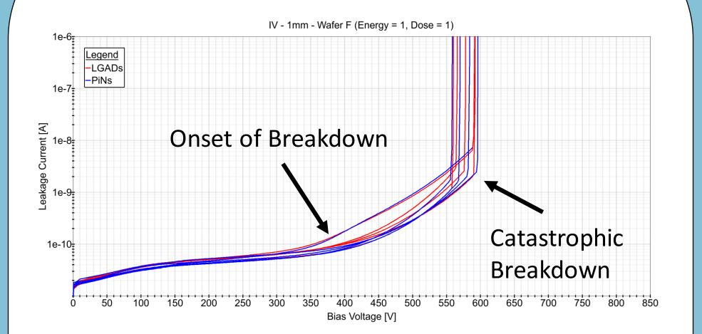
Example IV curves for 1mm devices of a single wafer type. For 1mm devices there is little difference between LGADs and PiNs.
