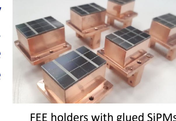
FEE holders with glued SiPMs
