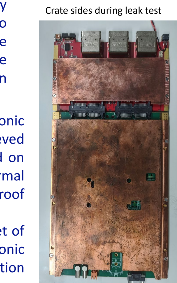
MB and Dirac coupled with copper plates
