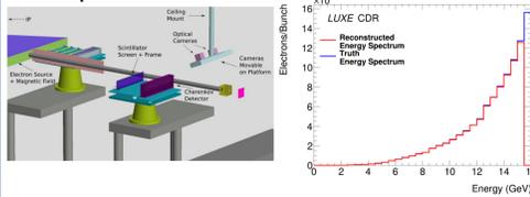
GEANT4 rendering of the electron detection subsystem
