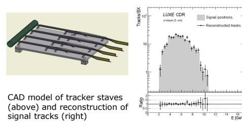
CAD model of tracker staves (above) and reconstruction of signal tracks (right)
