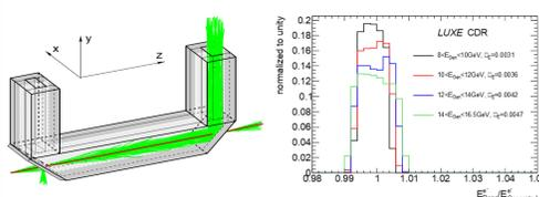
GEANT4 rendering of Čerenkov prototype (left) and reconstruction of electron energy (right)
