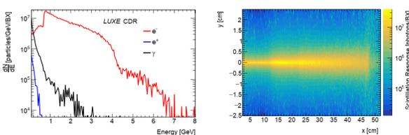
Simulated energy spectra at spectrometer scintillator plane
