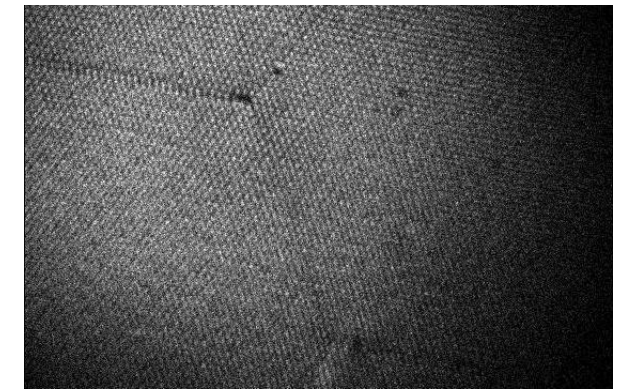
Close-up of the nine-electrode pattern MCP pore limited image resolution
