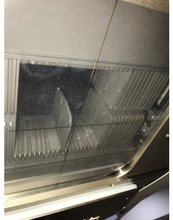
MLC with single leaf extended into field
