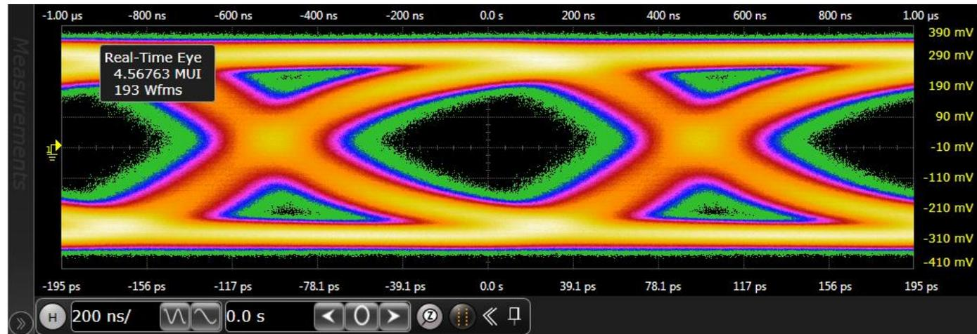
“Eye diagram” with transmitter at 5.12 Gbit/s
