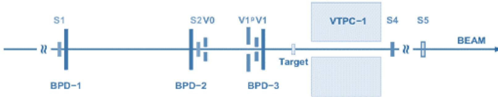
Beam Position Detectors (BPD-1,2,3) provide position and charge measurement of the incoming beam particles during the data taking.
