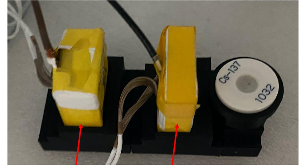
Absorber (Thickness 3 mm) Scatterer (Thickness 3 mm)
