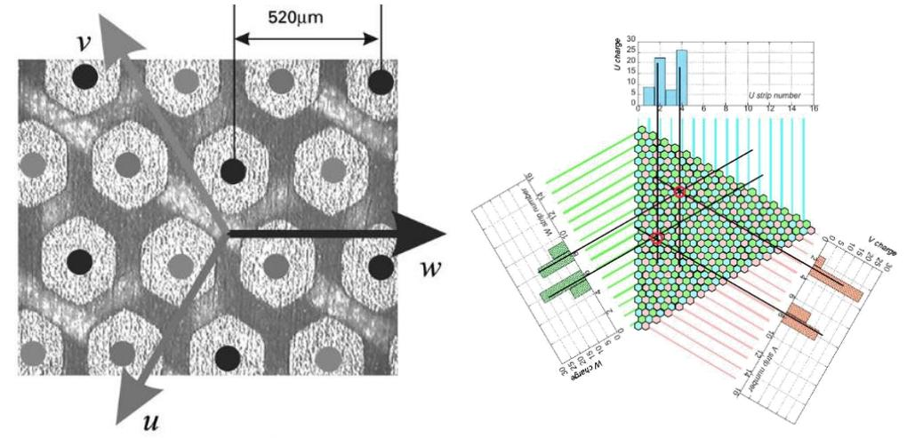
Fig. 4. Microscope photograph of the novel micropad readout. The micropads are alternately connected to three different layers of strips.
