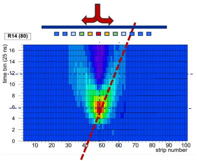
Figure 4. Intensity plot of ADC counts in the R14 chamber plotted against strip number on the horizontal axis and the time bin number (25 ns) on the vertical axis.
