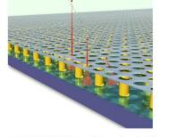
Fig. 1. The InGrid detector. Electrons from the drift volume cause an avalanche in the gap between the pixel chip and the grid.
