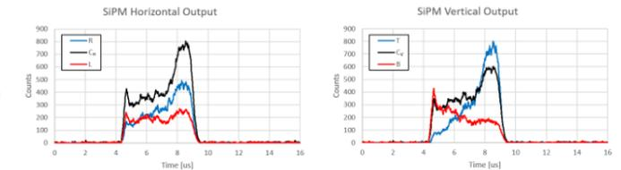
Figure 8. The  $\alpha$ -induced LG-SiPM signals from the  $x$  axis channels  $L$ ,  $C_H$  and  $R$  (left) and  $y$  axis channels  $T$ ,  $C_V$  and  $B$  (right). This event was recorded at a  $V_{bias}$  of  $-34$  V. The origin of the time axis corresponds to the global event trigger as discussed in Section 2.6.
