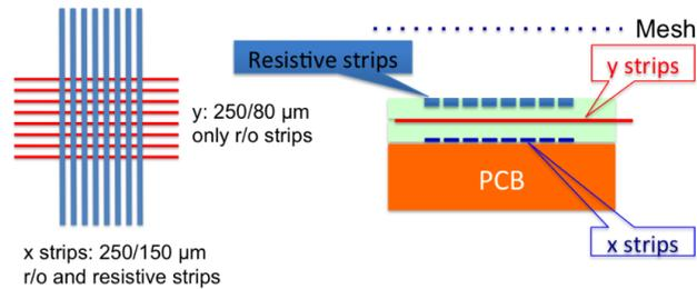
Figure 2. X-Y chamber schematics. Left. Strip layout. The bottom X readout strips are parallel to the resistive strips. The Y strips are at 90°. Right. Vertical cross-section. The X readout strips and the resistive strips are going into the figure.
