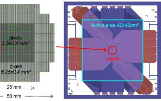
Figure 2: Sketch of large pixelized Micromegas detector (right). Zoom of the pixel area (left)
