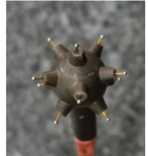
Additionally, it is possible to read out each anode individually, allowing the three-dimensional reconstruction of the ionisation tracks.
