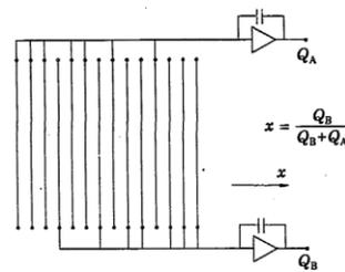
Figure 3.2.3: Graded Density Cathode
