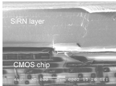
Fig. 3. Cross section SEM picture of a Timepix chip covered with 9 μm SiRN.
