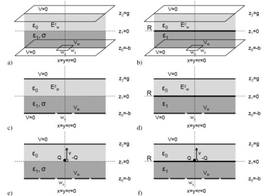
Figure 30. Weighting field for a geometry with a resistive layer having a bulk resistivity of  $\rho = 1/\sigma$  [ $\Omega\text{cm}$ ] (left) and a geometry with a thin resistive layer of value  $R$  [ $\Omega\text{cm}^2$ ] (right).
