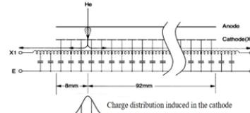
Fig. 8. Equivalent circuit of the delay-line PPAC detector.
