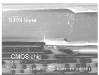
Fig. 3. Cross section SEM picture of a Timepix chip covered with 9 µm SiRN.
