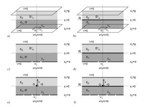
Figure 30. Weighting field for a geometry with a resistive layer having a bulk resistivity of  $\rho = 1/\sigma[\Omega cm]$ (left) and a geometry with a thin resistive layer of value  $R[\Omega/\text{square}]$  (right).
