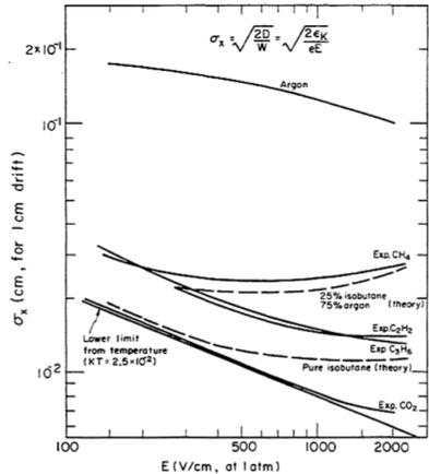
Fig. 35 Computed and experimental dependence of the standard deviation of electron diffusion from the electric field for 1 cm drift, in several gases at normal conditions<sup>25)</sup>
