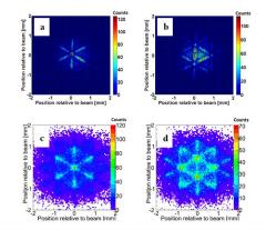
Figure 10. Reconstruction of the points of interaction, from the center-of-gravity of the light emitted from several holes, when irradiating at THGEM type 1, configuration go (table 3) at the center of a hole and inbetween holes. a) and b) are experimental results (with 8 keV x-rays) at gain 10<sup>4</sup>; c) and d) are simulation results (with 8 keV electrons). See text for explanations of the figures, and section 2.3.3 for explanations of the experiment and simulation.
