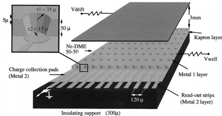
Fig. 1. Schematic diagram of a WELL detector.
