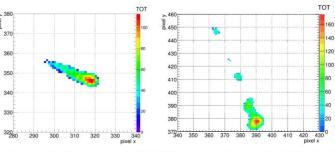
Figure 15. Examples of particle tracks measured with the GEMPix: a proton track (from neutron irradiation) with a visible increase in the energy deposition towards the end of the track (left) and an electron track (from <sup>137</sup>Cs irradiation, right).
