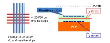
Figure 2. X-Y chamber schematics. Left. Strip layout. The bottom X readout strips are parallel to the resistive strips. The Y strips are at  $90^{\circ}$ . Right. Vertical cross-section. The X readout strips and the resistive strips are going into the figure.
