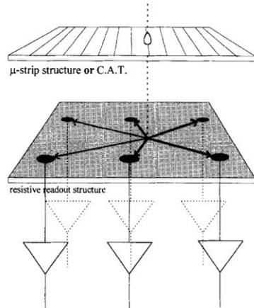
Fig. 1. 2D resistive charge division – schematic.
