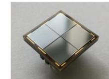
Figure 7. The  $2 \times 2$  array of LG-SiPMs used in these studies. Power and readout are provided by a separate PCB that attaches to the underside of the array via a pin-socket.
