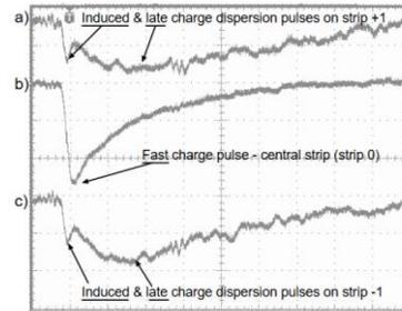
Fig. 4. Observed charge dispersion signals on three adjacent strips for a single x-ray photon conversion in the double-GEM detector. Tikronix scope pulses with 400 ns/div on the a) right strip (20 mV/div), b) central strip (50 mV/div) and c) left strip (20 mV/div).
