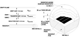
Fig. 1. Schematics of the resistive anode double-GEM detector used for charge dispersion studies.
