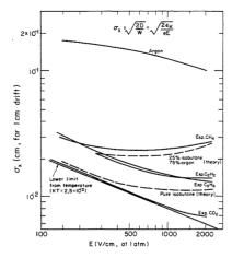
Fig. 35 Computed and experimental dependence of the standard deviation of electron diffusion from the electric field for 1 cm drift, in several gases at normal conditions<sup>25</sup> F.Sauli, Principles of operation of multiwire proportional and drift chambers, CERN, 1977 (https://cds.cern.ch/record/117989)
