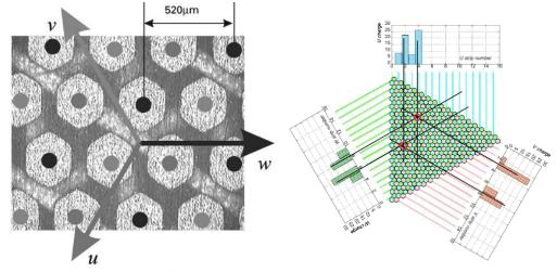
Fig. 4. Microscope photograph of the novel micropad readout. The micropads are alternately connected to three different layers of strips.
