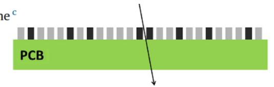
Fig. 4. Principle of the genetic multiplexing. A particle (array) leaves a signal on two neighbouring strips which are connected to two given channels. These channels are connected to other, non-neighbouring strips in the detector. The recorded signals on these two channels therefore localize without ambiguities the particle in the only place where strips are consecutive.
