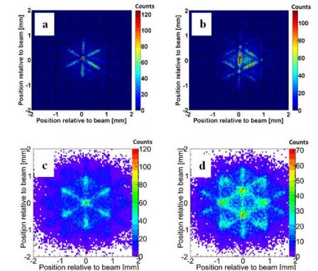
Figure 10. Reconstruction of the points of interaction, from the center-of-gravity of the light emitted from several holes, when irradiating a THGEM type 1, configuration g (table 3) at the center of a hole and in-between holes. a) and b) are experimental results (with 8 keV x-rays) at gain  $10^4$ ; c) and d) are simulation results (with 8 keV electrons). See text for explanations of the figures, and section 2.3.3 for explanations of the experiment and simulation.
