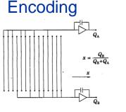
Figure 3.2.3: Graded Density Cathode
