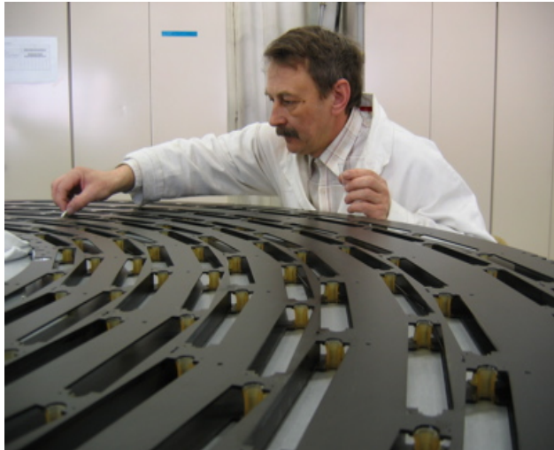
Tracker Support Tube and Thermal Screen being Prepared for Commissioning
