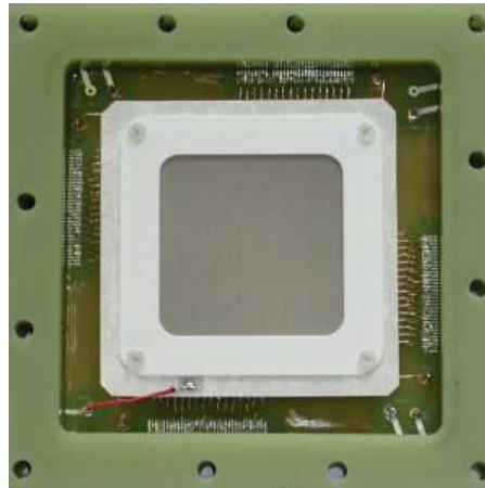
Fig. 1. Inner components of the MicroCAT detector with its interpolating readout structure. The cylindric pin spacers are fixed on the readout nodes.
