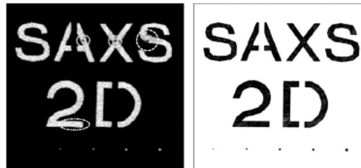
Fig. 18. On the left-hand side the image of the "SAXS" aperture recorded with a PCB-readout structure is shown. On the right-hand side a photo of the aperture taken with a standard digital camera against the sunlight is depicted. The distance between detector and source amounted to about 2.5 m, therefore parallax is very small. The illuminated spots at the bottom correspond to holes in the aperture with diameters of 280, 380, 480, 580 and 680 \mu\text{m} . The aperture is slightly tilted by an angle of about 0.6^\circ , which can be recognised for example by the vertical pixel jump (pixel quantisation) at the bottom of the "2" (dashed-dotted line). The sizes of both depicted images amount to 4.4 \times 4.4 \text{ cm}^2 .
