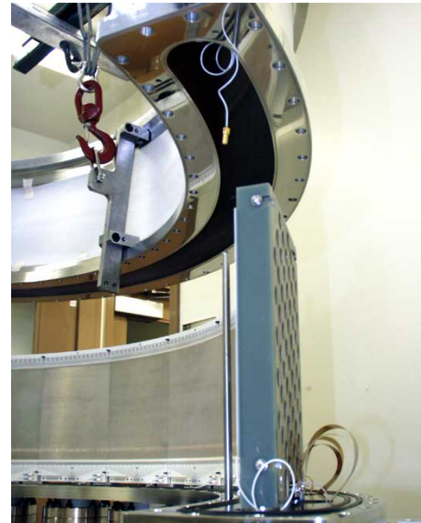
Pressure vessel being lowered
