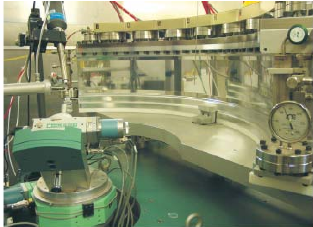
Figure 1. The Protein Crystallography Station at the Los Alamos Neutron Science Center. The sample is held by the rotating stage at the bottom left. Eight detectors are arrayed about 1 meter away from the sample to collect the scattered neutrons. (Courtesy of Gery Bunick.)
