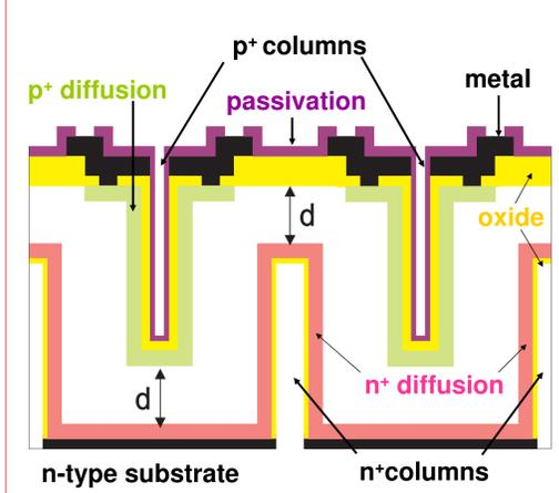
**Technology simplification of DDTC with respect to full 3D:**
