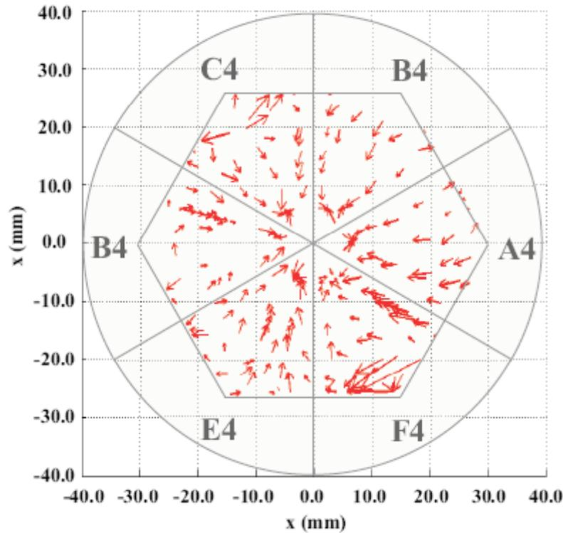
a) Displacement vectors,  $z = 4.8 \pm 0.3 \text{ mm}$
