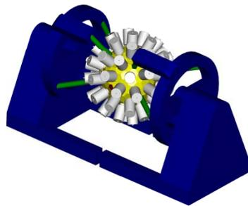
Completed array (6480 segments) with support structure
