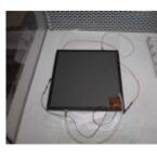
All RPCs are tested in streamer mode. Discriminator threshold for the RPC signal is set at -40 mV.
