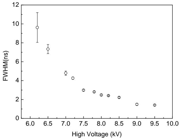
Fig. 8. The time resolution as a function of HV for a silicone coated P-120 grade bakelite RPC.
