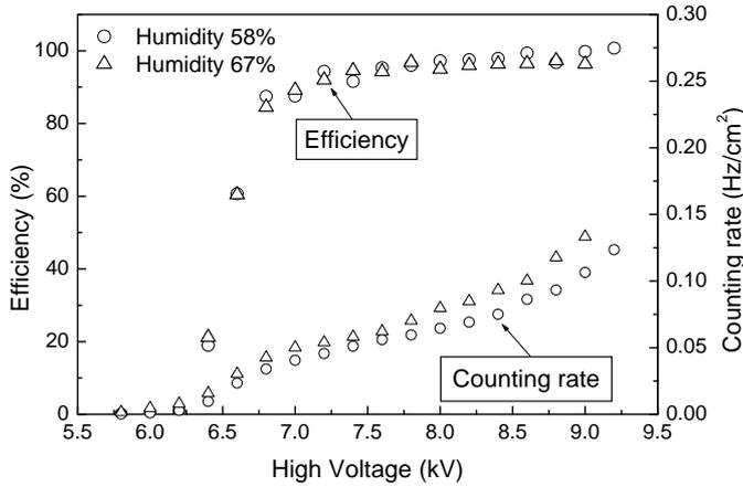
Fig. 4. The efficiency and the counting rate versus high voltage for different humidities for a silicone coated P-120 grade bakelite RPC.
