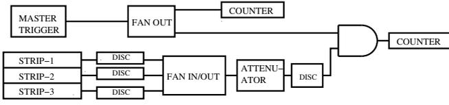
Fig. 1. Schematic representation of the crosstalk measurement setup, as mentioned in Ref 7.
