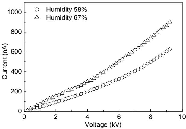
Fig. 5. Current versus high voltage for different humidities for a silicone coated P-120 grade bakelite RPC.
