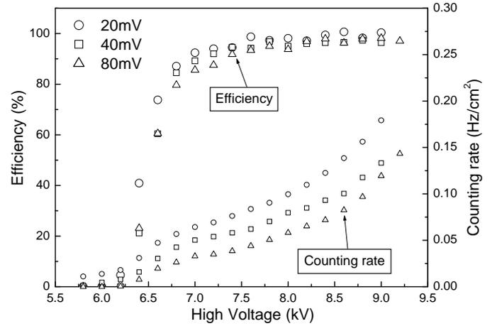
Fig. 2. The efficiency and the counting rate as a function of high voltage for a silicone coated RPC made of P-120 grade bakelite with discriminator threshold values of 20 mV, 40 mV and 80 mV. Used gas mixture is Argon (34%) + Isobutane (7%) + R-134a (59%).
