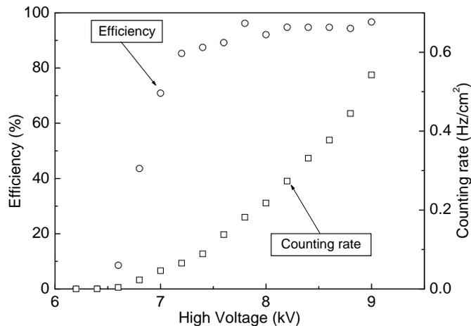
Fig. 9. The efficiency and the counting rate as a function of HV for uncoated P-120 grade bakelite RPC.
