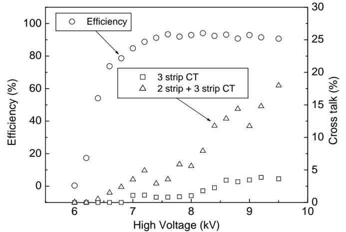
Fig. 7. Variation of the crosstalk with the high voltage in comparison with the efficiency for a silicone coated P-120 grade bakelite RPC.
