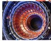
Inner Tracker (barrel-TIB, disks-TID)
