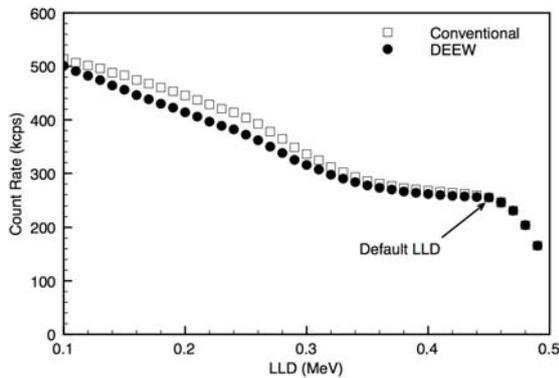
Fig. 3. True count rates with different LLDs of the DEEW and conventional energy window methods.
