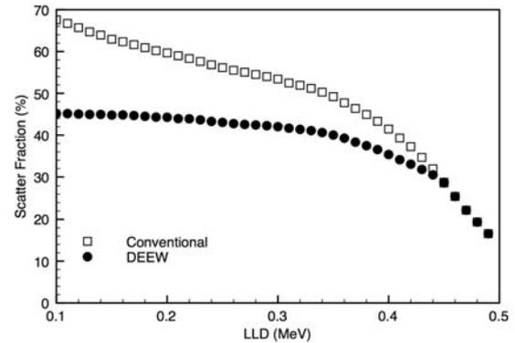
Fig. 4. SF with different LLDs of the DEEW and conventional energy window methods.
