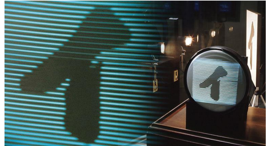
The Japanese character “イ” displayed on a cathode-ray tube. (The photograph shows a device reproducing the character in the Hamamatsu Science Museum.)
