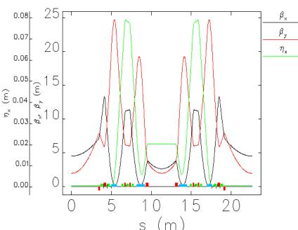
This lattice originated the modification of the existing cell2 too a DDBA cell
