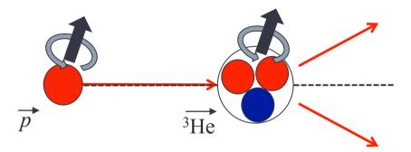
Spin correlation coefficient  $C_{yy}$  is obtained by bombarding the polarized proton beam on the polarized <sup>3</sup>He target and measuring the asymmetry of the scattered particles.
