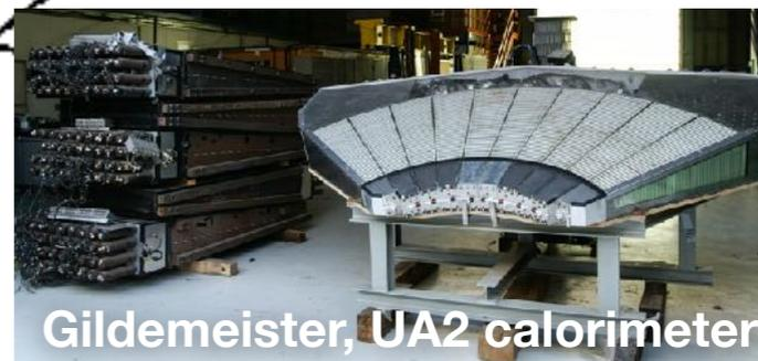
Performance: With em calorimeter, precise measurement of hadrons, jets, taus & missing transverse energy (ETmiss) w. jet resolution  $\sigma/E \sim 50\%/\sqrt{E}$  [GeV]  $\oplus$  3%, response linearity within  $\sim 1\%$  up to few TeV energies and good ETmiss.
