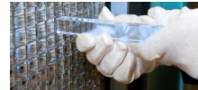
Insertion of lead-kgLuPb crystals (over three times the density of conventional glasses) into the high granularity electromagnetic calorimeter of the ALICE detector giving percent scale energy measurements. (© CERN)
