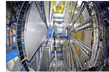
ATLAS gas detector based muon spectrometer, which covers a total area the size of a football field and measures the paths of the muons that pass through it to an accuracy of better than a tenth of a millimetre. (© CERN)
