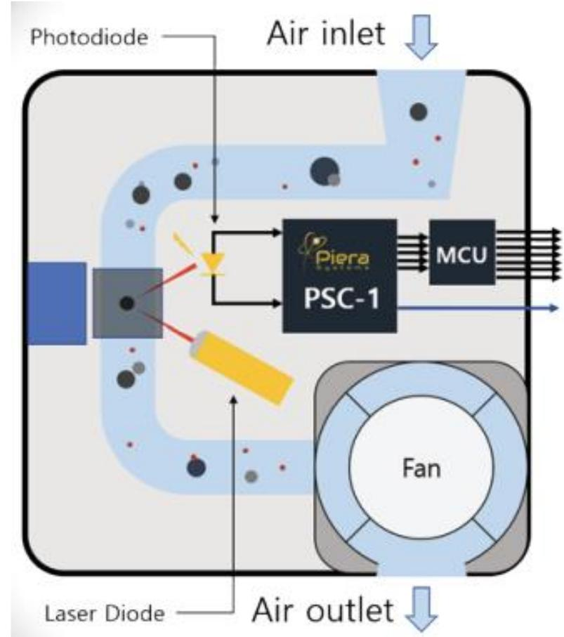
Based on a single photo-diode
