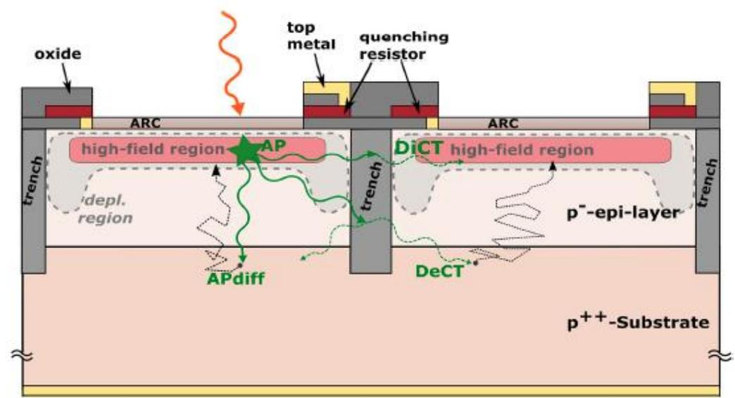
Fig. 1. Schematic representation of the internal structure of FBK Silicon photomultiplier, made in RGB-HD or RGB-UHD technology, with deep trenches between cells (SPADs).
