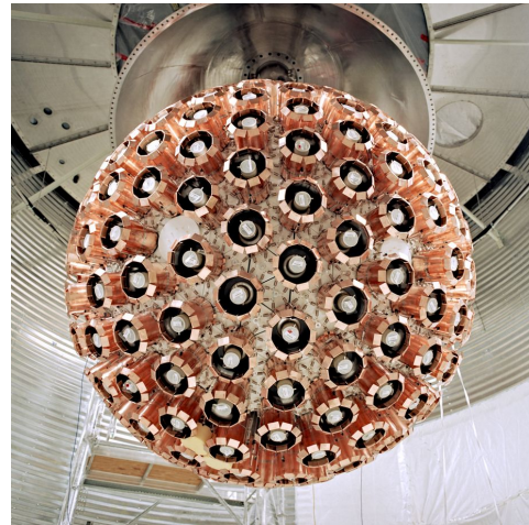
Acrylic Vessel With Copper Thermal Shorts
