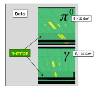
Why 1<sup>st</sup> layer of EM calorimeter is so finely segmented:
