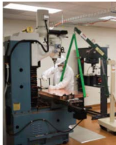
Copper being electroformed on a stainless steel mandrel
