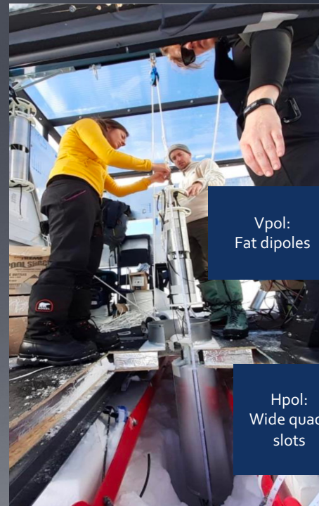
Deep channels lowered by hand
