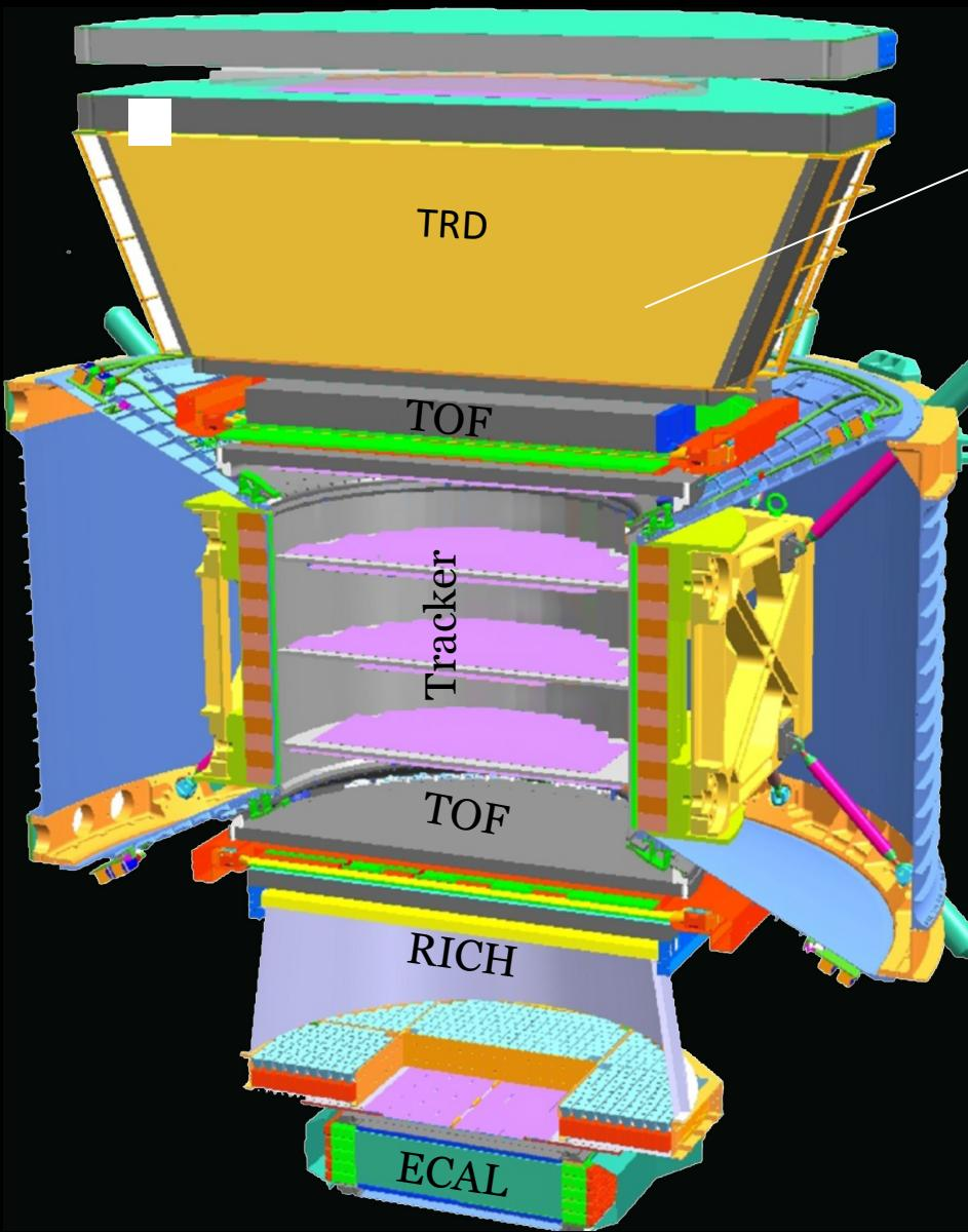
Transition Radiation Detector (TRD) separates  $e^\pm$  from protons using transition radiation measured in 20 layers of proportional tubes.
