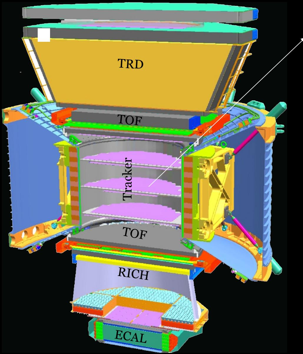
Silicon tracker and magnet distinguish between  $e^-$  and  $e^+$  up to a few TeV using 9 layers over 3 m lever of arm
