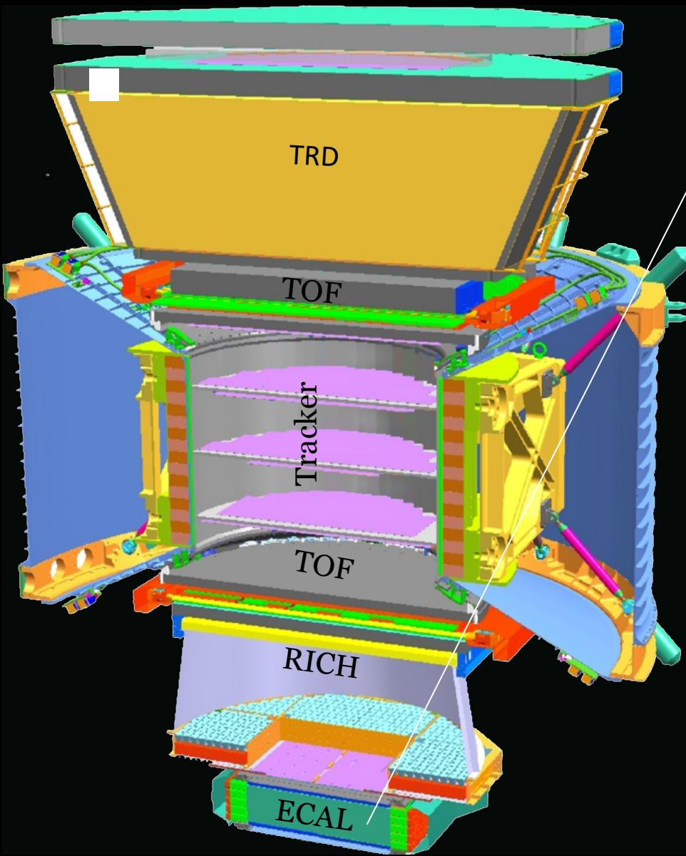
Electromagnetic Calorimeter (ECAL) provides a precision 3D measurement of energy and shower development over  $17X_0$
