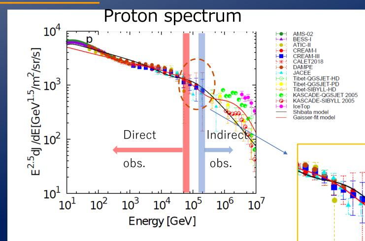
→ Proton measurement with large detection area using Tibet-III and MD
