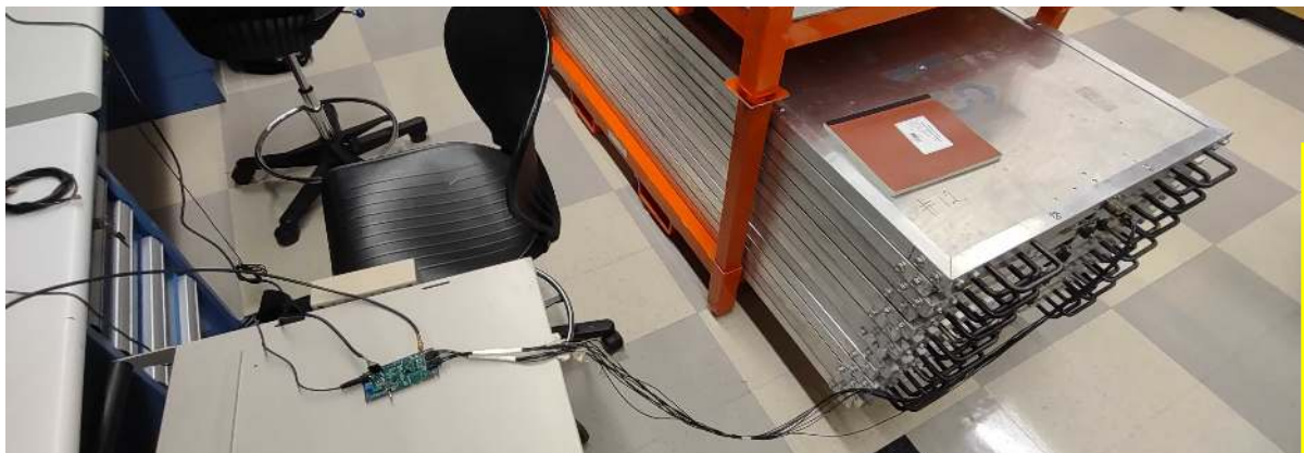
Dylan Frikken (OSU) performs system tests on scintillator panels (left) and readout electronics (above).
