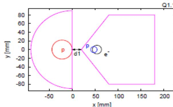
Figure 2: Transverse section of the first Q1 block showing the face closest to the IP.
