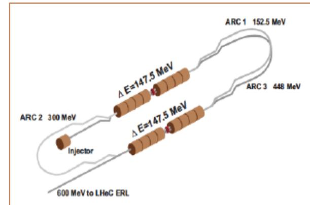
Figure 2: Consequent upgrade to LHeC pre-accelerator. By modifying the machine backleg to include a second full cryomodule, the recirculator can deliver higher beam energy of 600 MeV.
