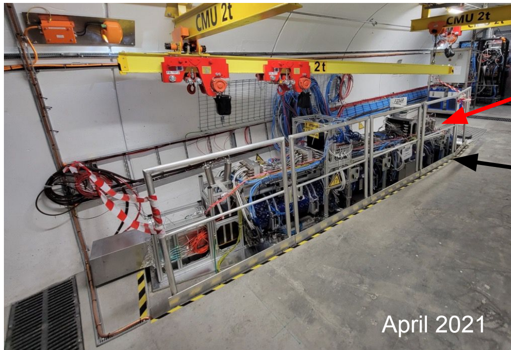
FASER spectrometer (magnets and tracker), trigger scintillators and calorimeter
