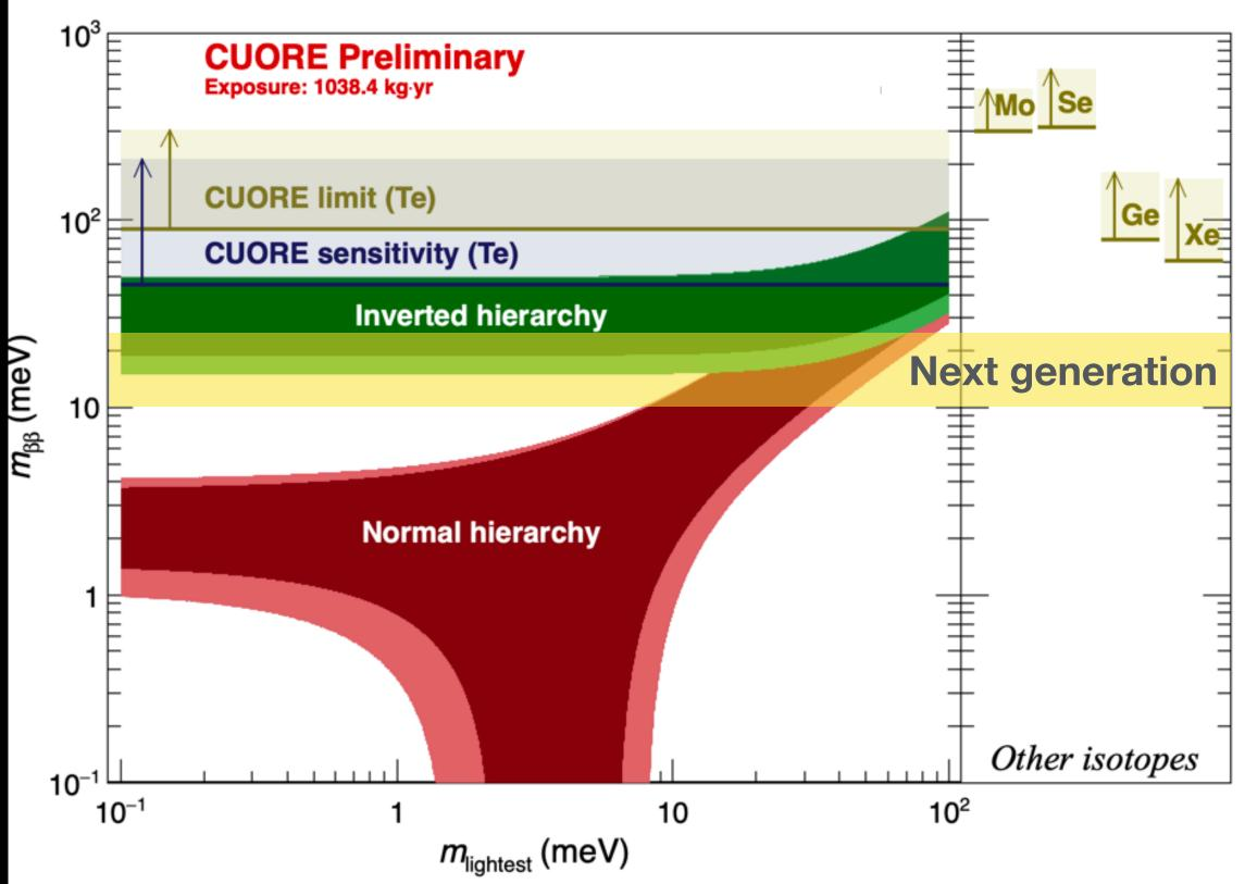
Oscillation parameters from <u>NUFIT 2020</u> are used. All limits are at 90% C.L. and 3 $\sigma$  uncertainty is shown on the inverted and normal hierarchy bands. The CUORE combined limit is now  $\langle m_{\mu\nu} \rangle < 90 - 305$  meV. The sensitivity line corresponds to the one quoted in the CUORE 2017 EPJC sensitivity paper. The limits on Ge, Mo, Se and Xe come from Gerda (2020), CUPID-Mo (2021), CUPID-0 (2019) and KamLAND-Zen (2016) respectively.
