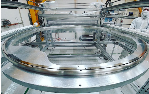
HV wire electrode grids woven at SLAC
