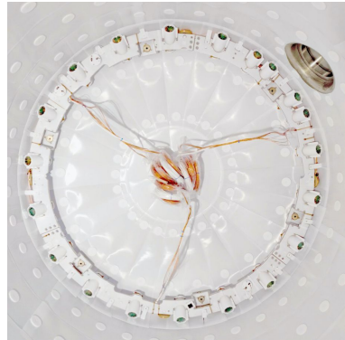
20 Bottom side dome PMTs in the ICV
