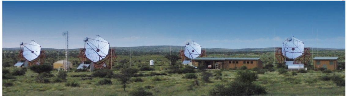
4 telescopes each of  $108 \text{ m}^2$  aperture
