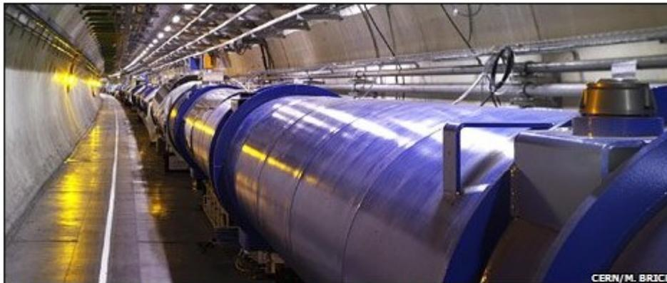
Superconducting magnets are cooled down using liquid helium
