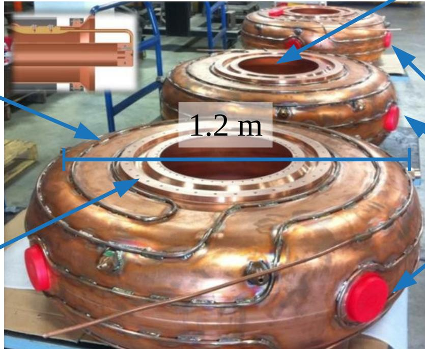
Internal surfaces treated to suppress breakdown
