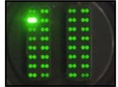
**Extruded plastic (PVC) cells filled with 10.2 million litres of scintillator instrumented with  $\lambda$ -shifting fibre and APDs**
