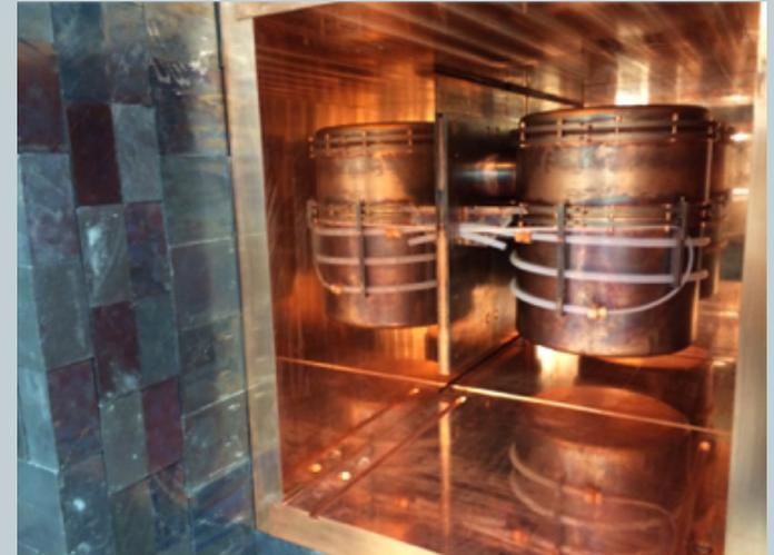
Modules 1 & 2 in Pb and Cu shielding
