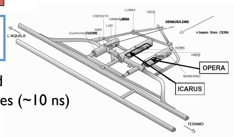
**OPERA:** a deep underground detector with charge and momentum reconstruction and excellent timing capabilities (~10 ns)
