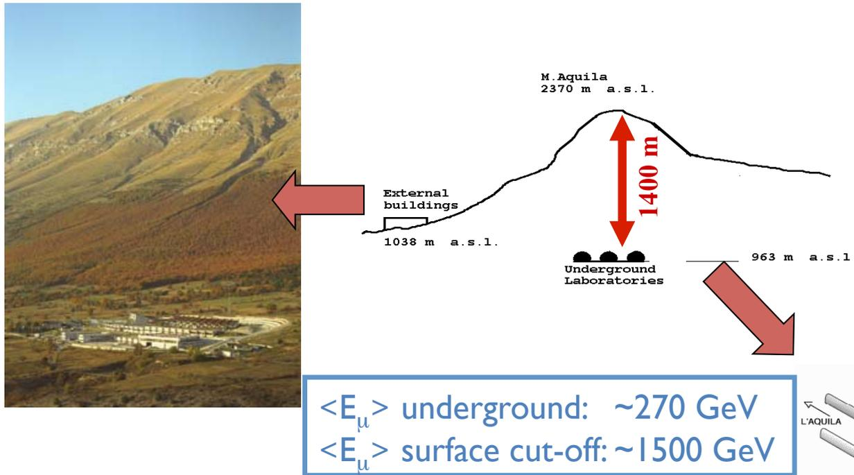
**Gran Sasso underground lab:** 1400 m of rock (3800 m.w.e) shielding, cosmic ray flux reduced by a factor  $10^6$  w.r.t. surface
