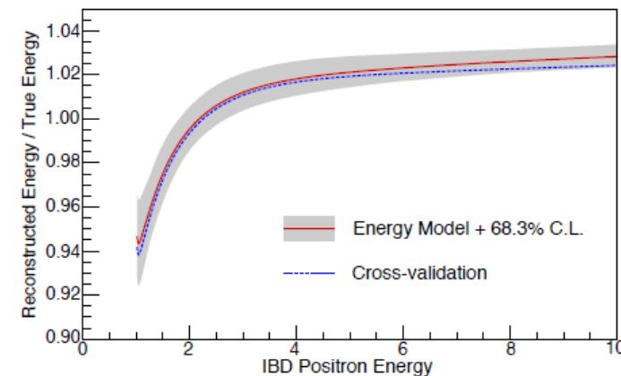
**Nominal energy model:** fit to mono-energetic gamma lines and  $^{12}\text{B}$  beta-decay spectrum
