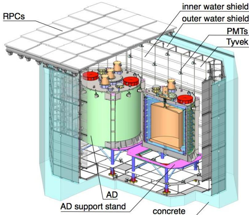
Two-zone ultrapure water cherenkov detector
