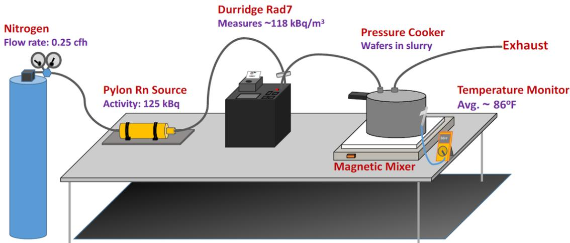
$^{210}\text{Pb}$  surface contamination during polishing insignificant  $\rightarrow$   $<1$  nBq/cm<sup>2</sup>
