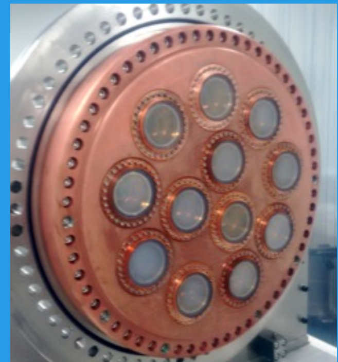
Energy plane 12 PMTs (Hamamatsu R11410-10) 30% coverage
