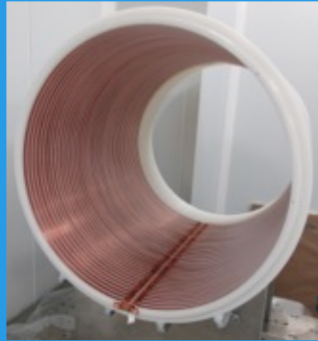
Time projection chamber 50 cm drift 20 cm radius
