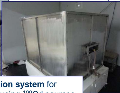
Radon-free calibration system for simultaneous calibration using  $^{109}\text{Cd}$  sources
